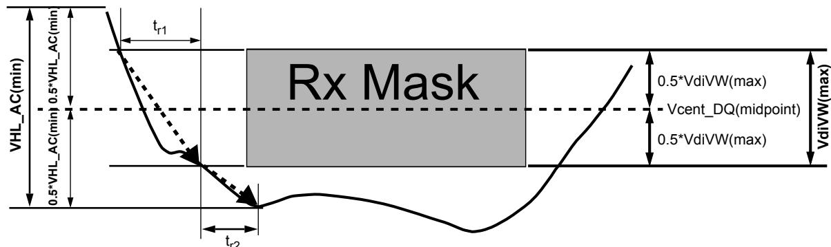
Figure 28. Slew Rate Conditions For Falling Transition
