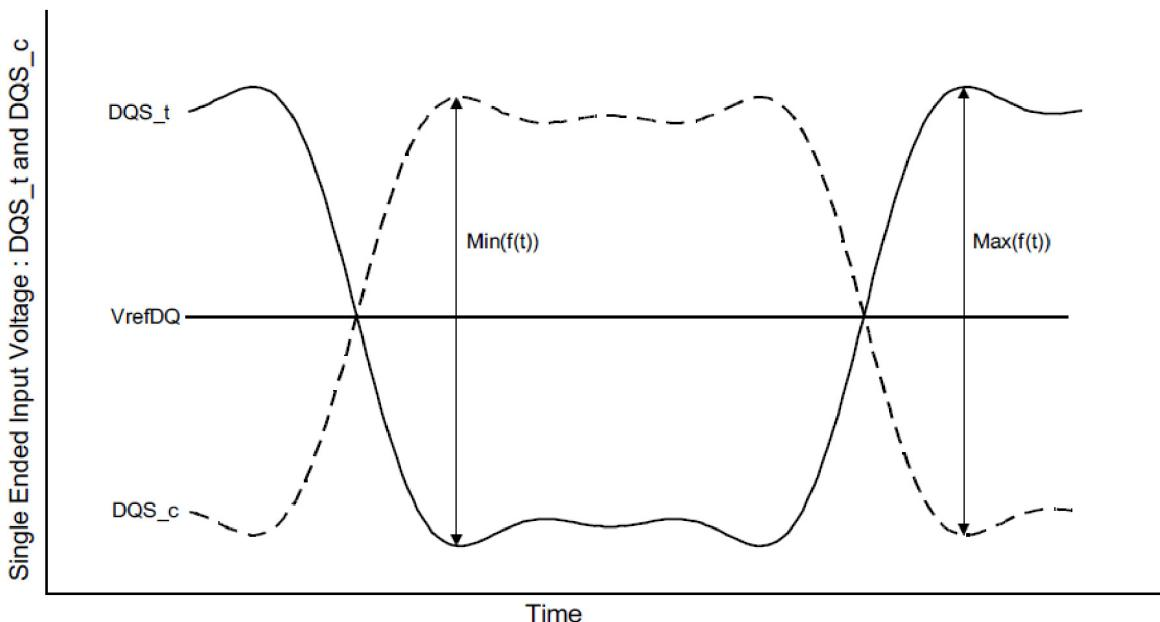
Figure 12. Definition of differential DQS Peak Voltage
