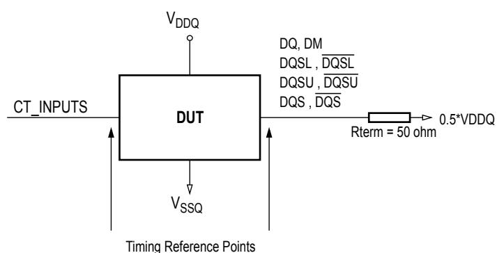
Figure 20. Connectivity Test Mode Timing Reference Load
