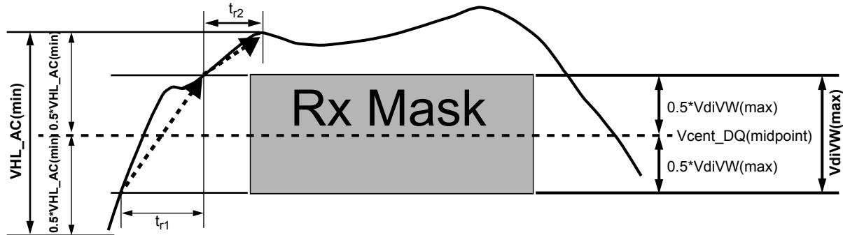
Figure 27. Slew Rate Conditions For Rising Transition
