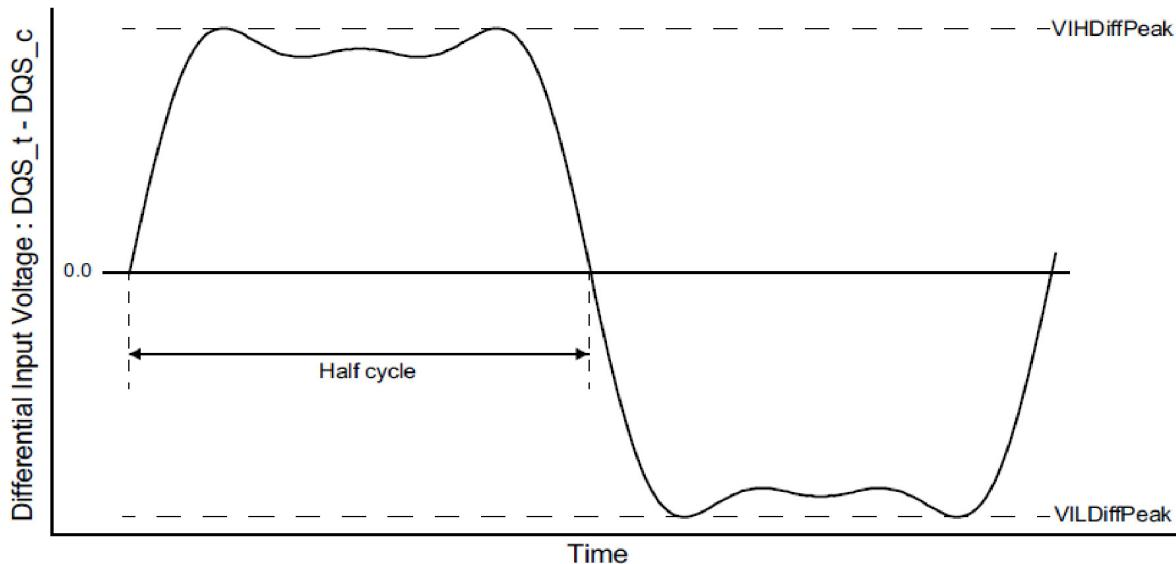
Figure 11. Definition of differential DQS Signal AC-swing Level
